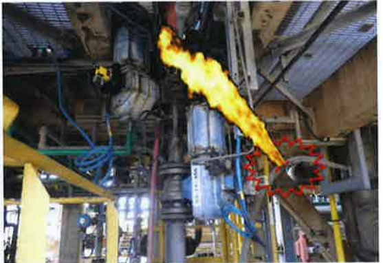
The flame affected to radioactive source of 08C108.
