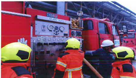
Fire truck driver discharge foam solution to 60D255 as required flow rate 1,750 gpm, discharge time 30 minute
